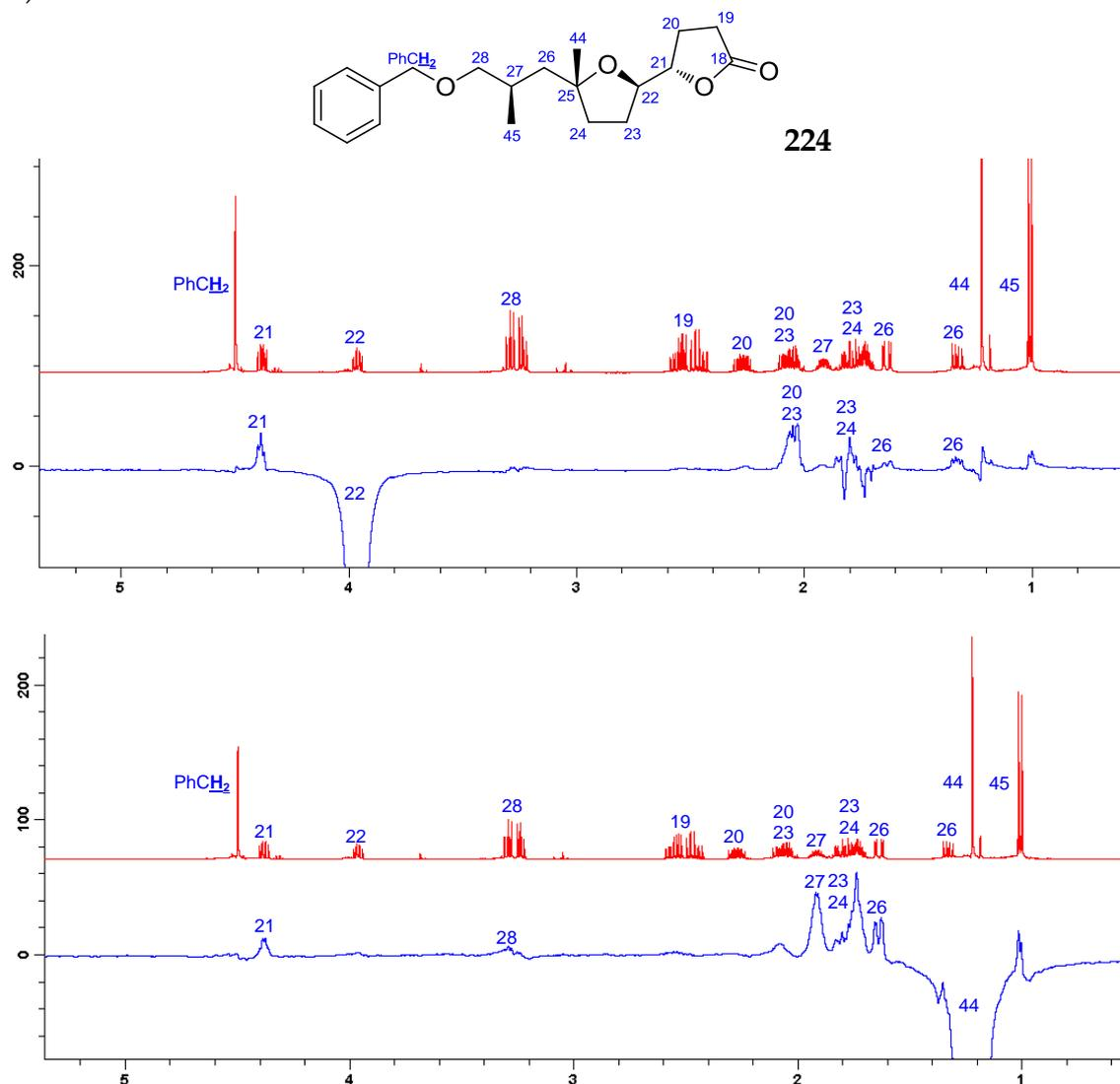
**Figure 26.** a) NOESY spectrum of compound **224**. b)  $^1\text{H}$  DPGFSE-NOE experiments with irradiation at 1.21 and 3.95 ppm. The key NOE-cross peaks of **224**.
