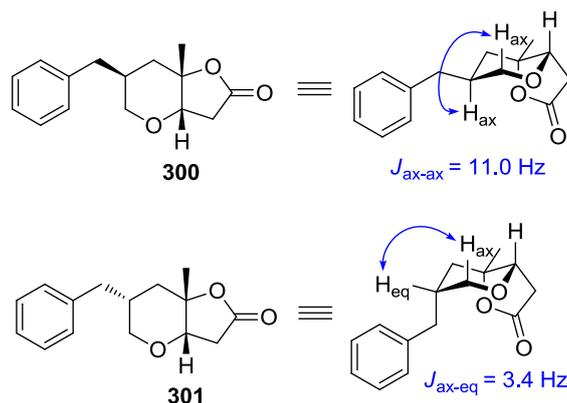
**Scheme 56.** Conformational drawings of (3*aS*,6*S*,7*aS*)-6-benzyl-7*a*-methylhexahydro-2*H*-furo[3,2-*b*]pyran-2-one (**300**) and (3*aS*,6*R*,7*aS*)-6-benzyl-7*a*-methylhexahydro-2*H*-furo[3,2-*b*]pyran-2-one (**301**).
