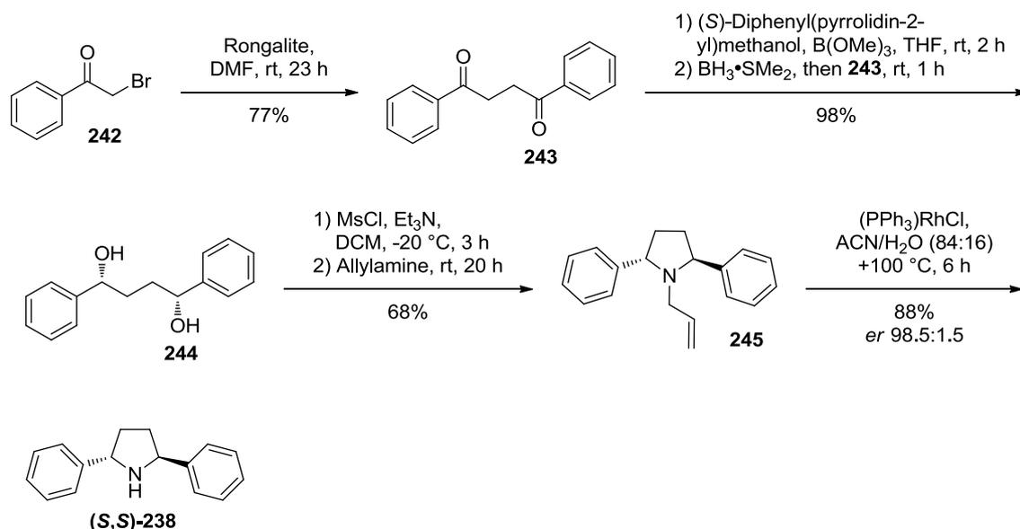
Scheme 38. Preparation of the (2*S*,5*S*)-diphenylpyrrolidine catalyst ((*S,S*)-**238**).<sup>95</sup>
