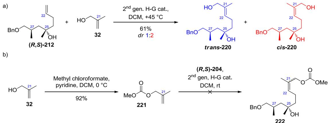
**Scheme 33.** Cross-metathesis reaction with a) methallyl alcohol (**32**) and b) the corresponding carbonate **221**.
