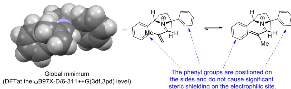
**Figure 17.** Possible structures of the catalyst-methacrolein iminium intermediates. Pyrrolidine ring of the formed iminium structure can have two different conformations: envelope and half-chair/twisted forms (only the envelope conformation is shown here). Additionally the methacrolein moiety can rotate; either methyl or methylene can point towards the phenyl group of the catalyst.
