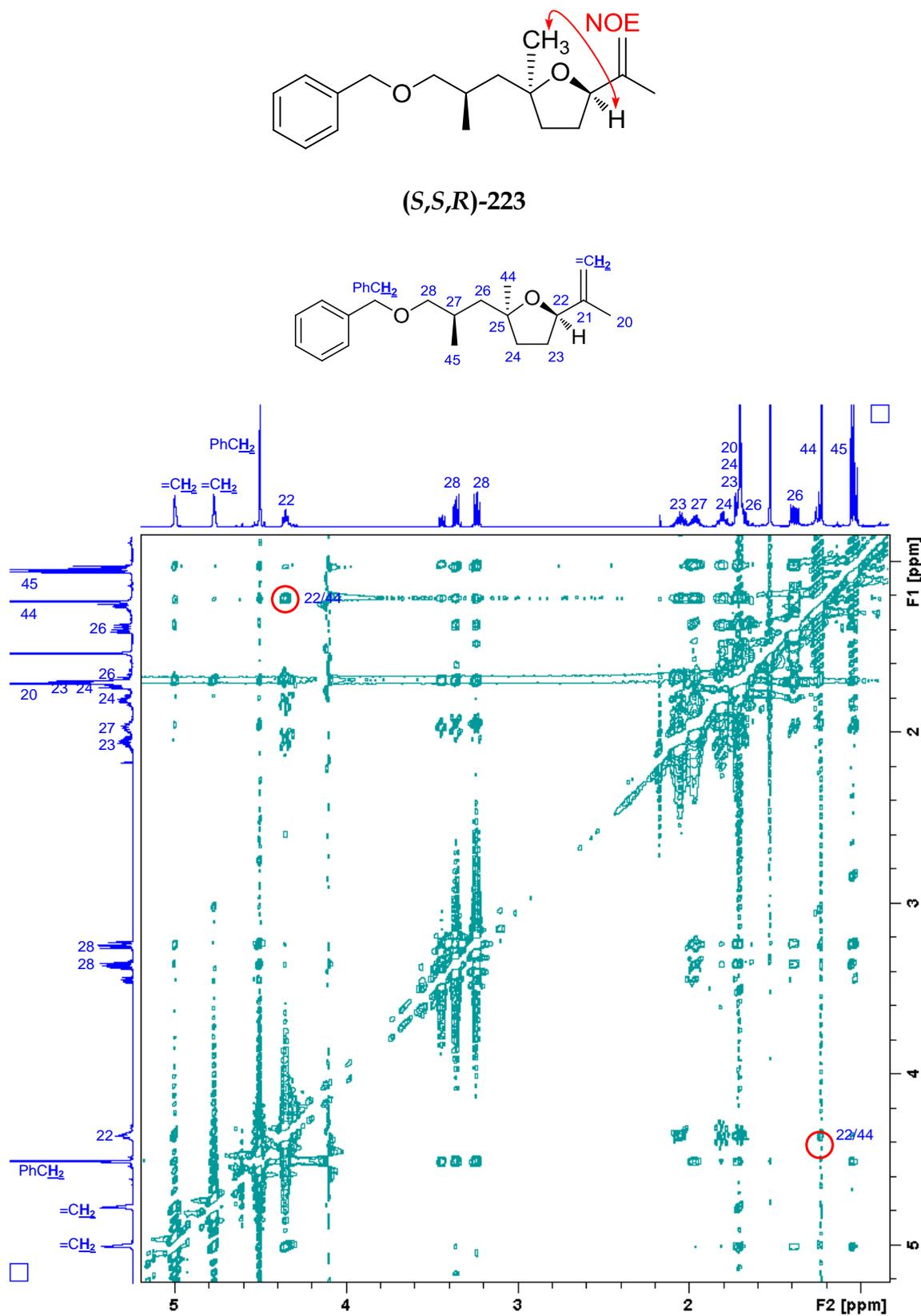
**Figure 25.** NOESY spectrum of the compound  $(S,S,R)$ -223, showing the correlation between 22H–44H and the lack of correlation between 26H–22H.
