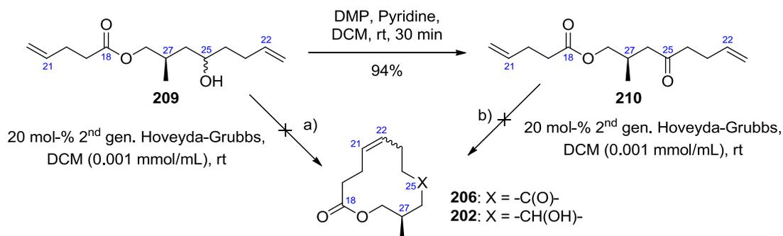
**Scheme 28.** Ring closing metathesis (RCM) for a) alcohol **209** and b) ketone **210**.
