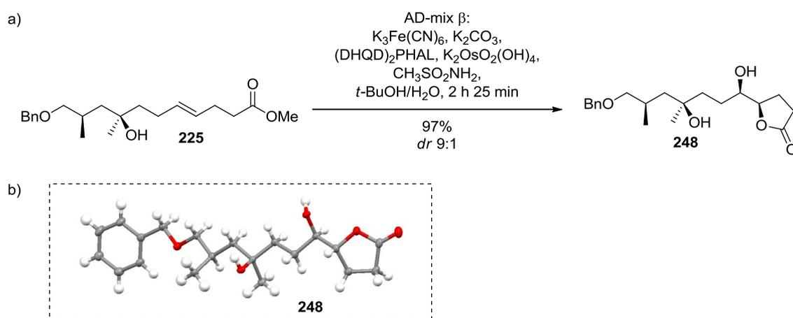
**Scheme 43.** a) The Sharpless asymmetric dihydroxylation reaction with AD-mix  $\beta$ . b) X-Ray structure of compound **248**.
