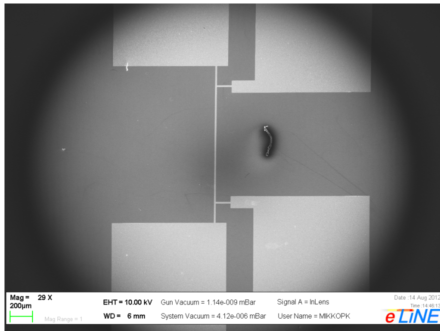
Figure 9: SEM image of a bismuth heater/thermometer deposited on \text{SiO}_x . The length of the line is 1 mm and the width is 10 \mu\text{m} .
