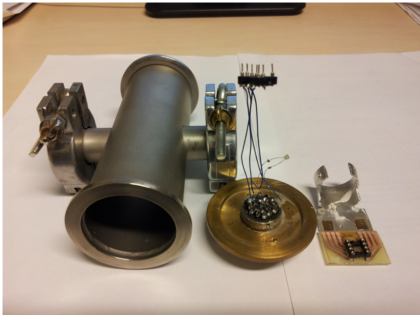
Figure 13: The vacuum chamber with the electrical feedthrough and the sample stage.
