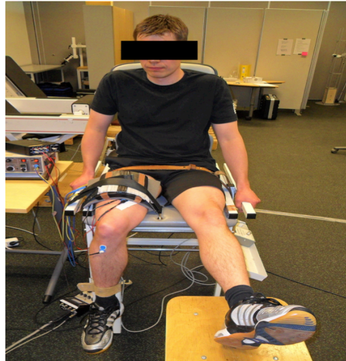
FIGURE 28. The electromechanical isometric knee extension device (designed and manufactured by the Department of Biology of Physical Activity, University of Jyväskylä) used to measure maximal isometric knee extension force during the assessment of voluntary activation through super-imposed muscle stimulation.
