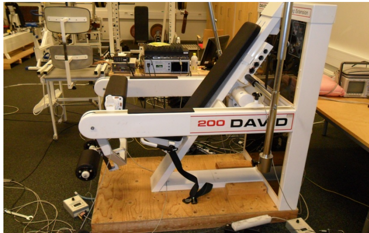
FIGURE 27. David 200 knee extension and flexion device used in the study (David Health Solutions Ltd, Helsinki, Finland) modified for isometric strength testing (Department of Biology of Physical Activity, University of Jyväskylä, Finland).
