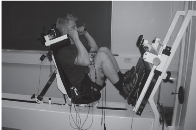
FIGURE 10 Modified M16 leg press device with mounted force plate and infra-red displacement sensor.
