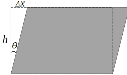
Figure 3.5: Shear characterized with angle \theta : \tan\theta = \frac{\Delta x}{h} .
