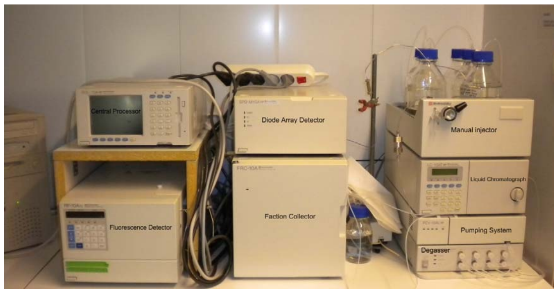
Figure 8 High Pressure Liquid Chromatography system used for sorting carbon DNA-CNT hybrids.
