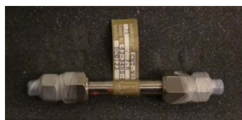
Figure 11 HYDROCELL CNT-NS 1500 column.
