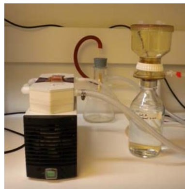
Figure 10 Filtering system used for purification of elution solutions that were used in IEX process.
