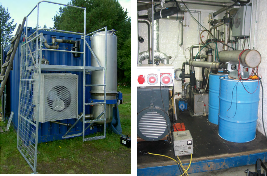
FIGURE 1. CENTRIA downdraft gasifier is based on patented EK gasification technology.
