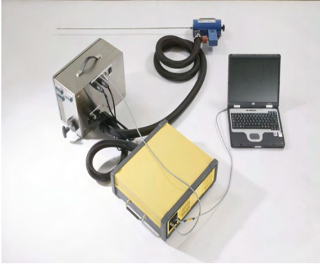
FIGURE 7. Centria R&D renewable energy laboratory FTIR gas analyser Gaset Dx4000N
