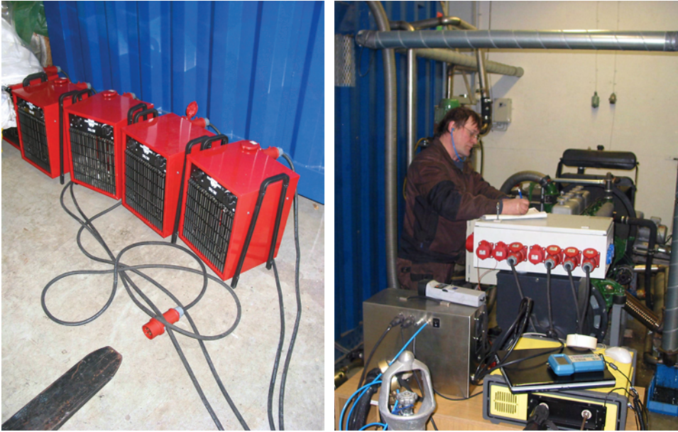
FIGURE 3. Study of the gas production and fuel consumption of the modified 8 litre 6 cylinder IC engine. Electrical power loads of 9 kW used in the experiment (left) and IC gas engine (right)
