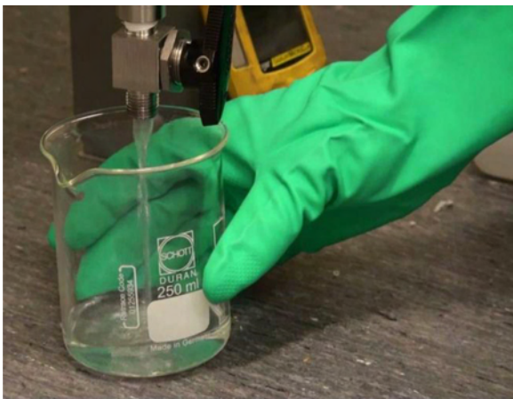
FIGURE 6. Methanol is drained from the facility, made from gasified black liquor.
