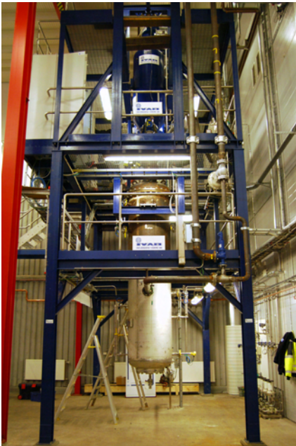
FIGURE 2. PEBG pilot plant at ETC (titled "IVAB gasifier") was put into operation in April 2011.
