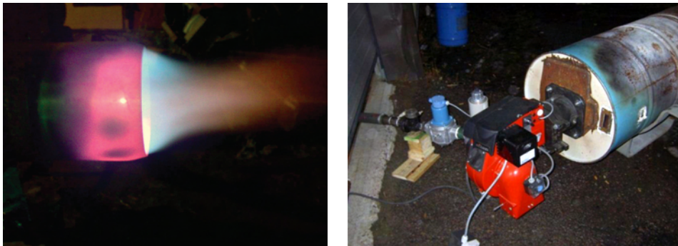
FIGURE 4. Evaluation of specific gas production using a gas burner. Wood gas fuelled gas burner (left) and test facility (right).
