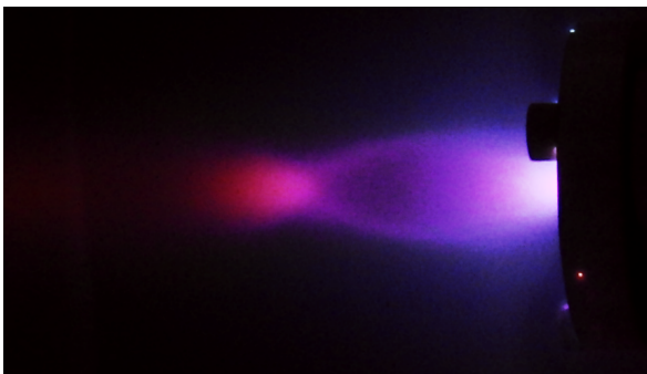
Figure 3.18: A photograph of an underexpanded argon jet that has a lower pressure difference compared to the jet in Figure 3.17. The gas cell pressure was 50mbar. The Mach disc size has reduced and is no longer present.
