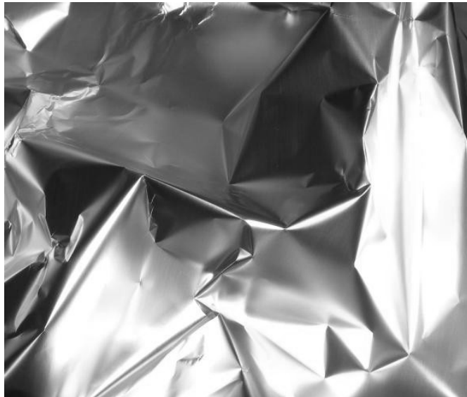
Figure 2.6: Loosely crumpled aluminium foil displaying a network of ridges meeting at sharp vertices.
