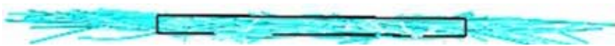
Figure 14. A side view of a fiber network for the adhesion force F_{ad} = 250 and the fiber stiffness k_b = 50 . The sheet thickness h is defined by the box that includes 80% of the fibers.
