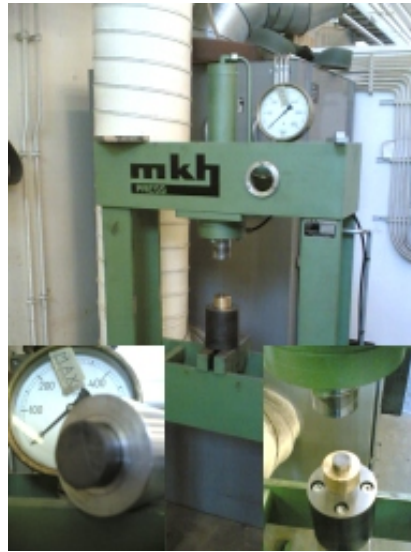
FIGURE B.2 It is non-trivial task to compress ^{13}\text{C} into a pellet. At JYFL a force of 30–50 kN has been put before it started to burn. The compressed pellet was supplied by undefined source in Russia protected by an industrial secret [65].
