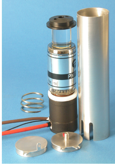
FIGURE 4.21 Photomultiplier tube with its constituents: quartz, FEU-187 and divider.
