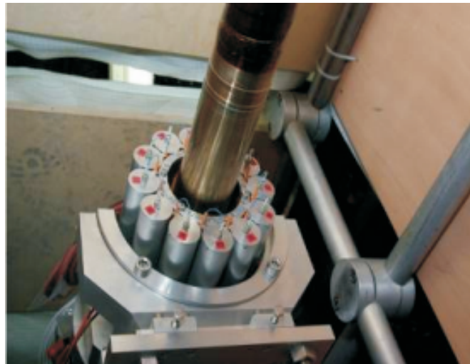
FIGURE 5.16 T0-A shortly after installation at ALICE Point 2.
