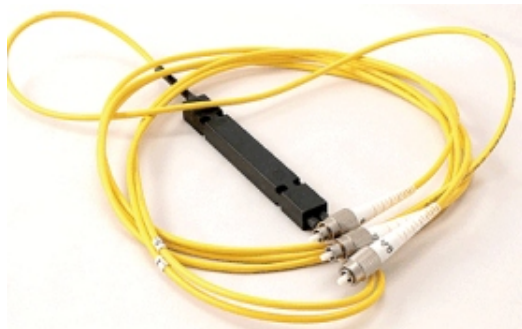
FIGURE 4.31 Optical splitter with a splitting factor 50/50 with fiber patchcords terminated with FC connectors [34]. Each splitting causes optical power dissipation of about 3 dB.
