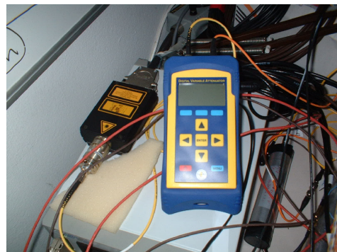
FIGURE 4.30 Integral parts of T0 LCS: Picoseconds' Injection Laser PIL040G (left) and Digital Variable Attenuator DA-100 [34] (right).
