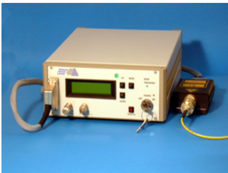
FIGURE 4.30 Integral parts of T0 LCS: Picoseconds' Injection Laser PIL040G (left) and Digital Variable Attenuator DA-100 [34] (right).
