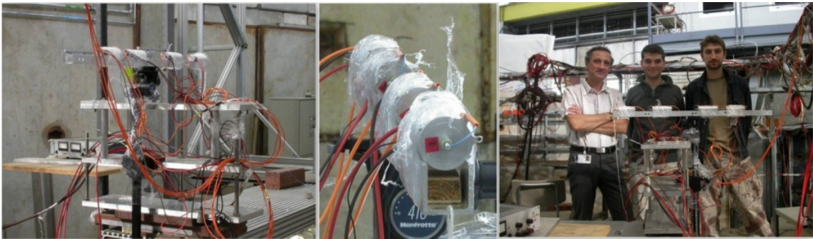
FIGURE A.7 Four T0 PMTs during the November 2005 full chain readout test at CERN.
