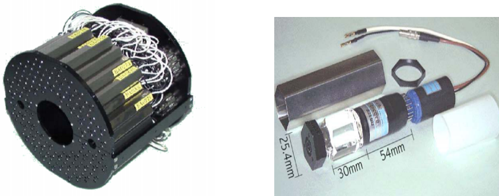
FIGURE A.2 Beam Beam Counter array at PHENIX (left). The outer diameter of the BBC is 30 cm and the inner diameter is 10 cm with clearance between the beam pipe and the BBC of 1 cm. A single BBC (right) consisting of 1 mesh-dynode photomultiplier tube mounted on a 3 cm quartz radiator.
