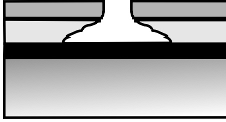
Figure 3.2: Undercut profile. From the bottom: silicon, SiO_2 , resist 1, resist 2.
