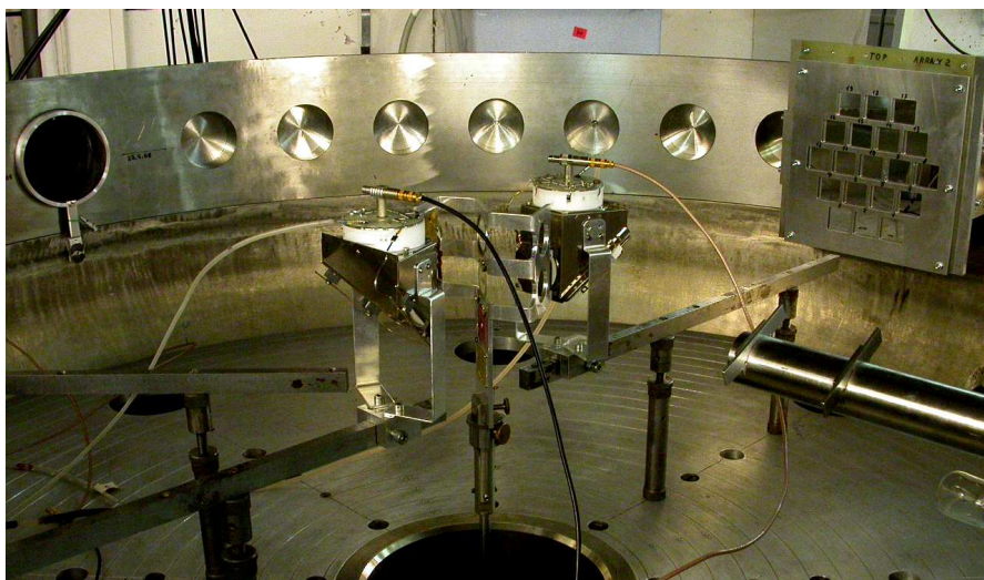
Figure 4.3 View of the experimental setup inside the reaction chamber. Only the right array of PIN detectors is seen.
